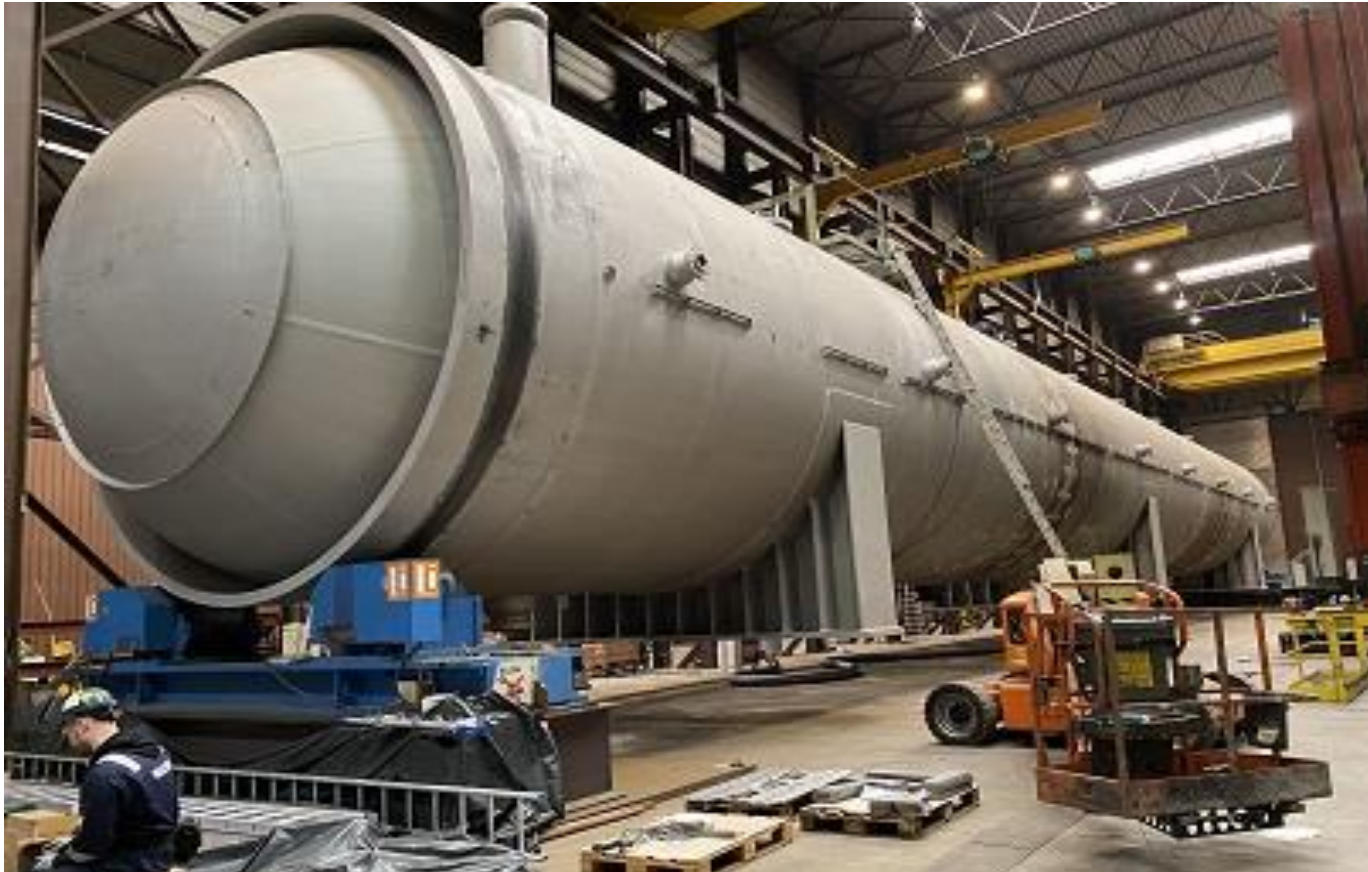
Length 50 m, diameter 6 m, weight 961 t
